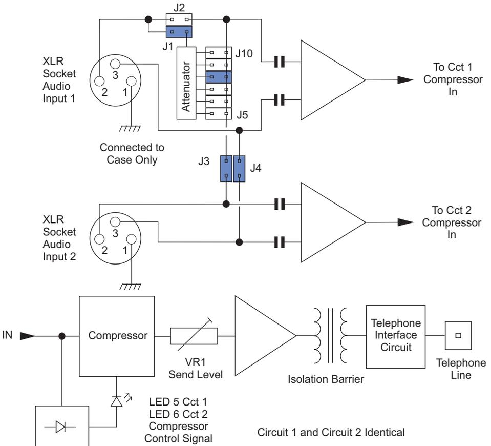
J4. If these links are NOT fitted, both circuits work independently but only circuit 1 has access to the attenuator circuit.
