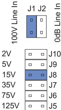
The TDS2 has two identical circuits which can be used totally independently of each other, or, can be tied together to share a single input. Circuit 1 has access to a 100V line attenuator, which can be shared by circuit 2. Note though that if both circuits are set to work independently of each other, then only circuit 1 has access to the attenuator.
